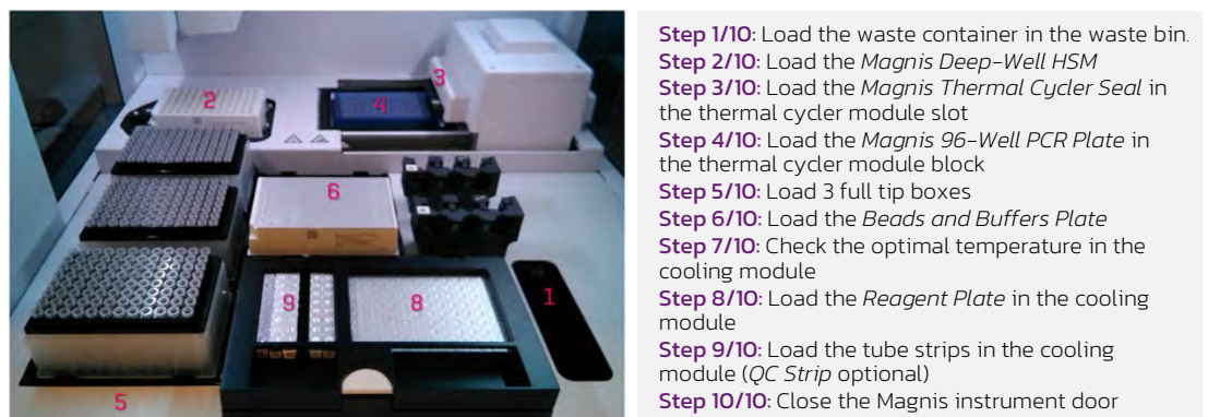
Figure 5. Magnis NGS Prep instrument deck loaded for the assay and quickloading guide.
